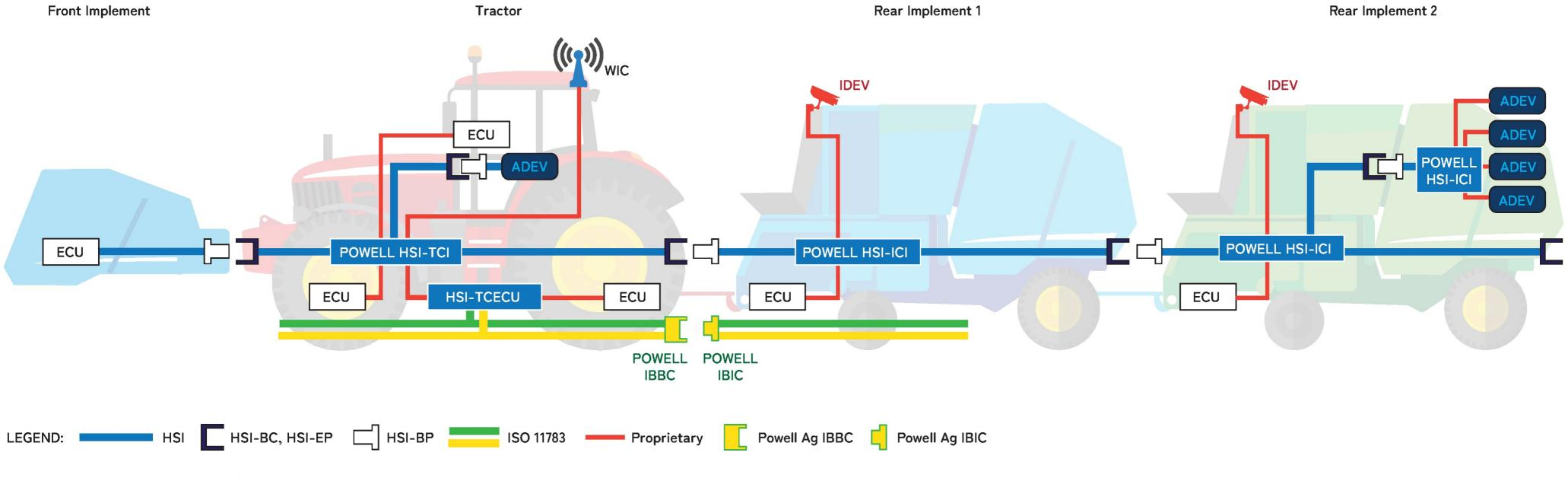
KEY: Powell HSI-TCI (Tractor Control Interface, Network Switch) | Powell HSI-ICI (Implement Control Interface, Network Switch) | ECU (Electronic Control Unit) | HSI-TECU (Gateway between tractor private network(s) and HSI) | IDEV (Integrated Device) | ADEV (Aftermarket Device) | WIC (Wireless Infield Communication Device)
